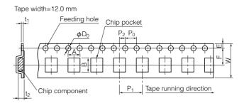
Taping condition: Lack of products in the middle of taping should be one MAX, but total quantity specified in the specifications should be secured.
