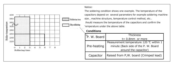
• The film capacitor has lower mounting heatresisting temperature than other capacitors, therefore the following cautions are needed.
