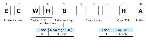
Rated voltage 800 V (Odd size taping)
