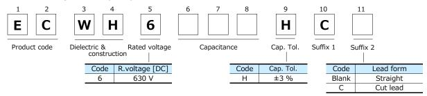
Rated voltage 630 V (Odd size taping)
