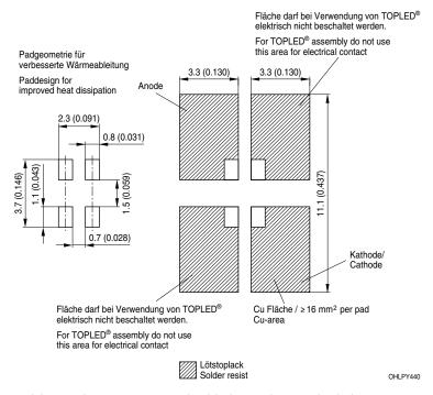
For superior solder joint connectivity results we recommend soldering under standard nitrogen atmosphere. Package not suitable for any kind of wet cleaning or ultrasonic cleaning.
