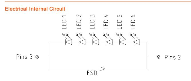
Pins 1: Substrate potential, isolated from Cathode and Anode Pins 2: Anode Ding 2: Cathode
