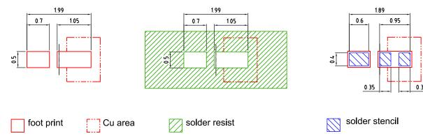
The usage of solder resist between anode and cathode pads is mandatory for applications where water may condense
