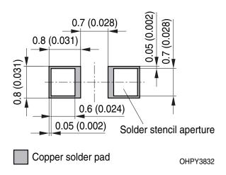
For superior solder joint connectivity results we recommend soldering under standard nitrogen atmosphere.
