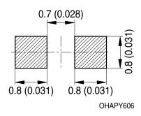
For superior solder joint connectivity results we recommend soldering under standard nitrogen atmosphere.
