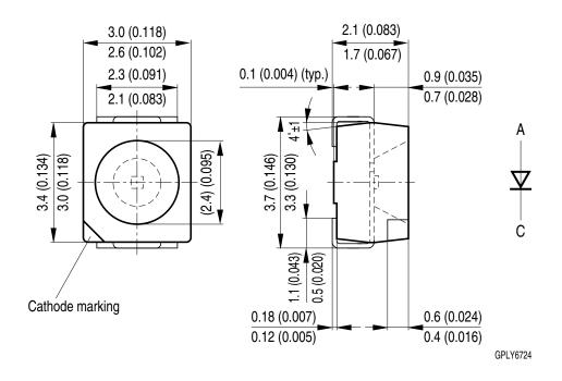
Approximate Weight:34.0 mgPackage marking:CathodeCorrosion test:Class: 3B
