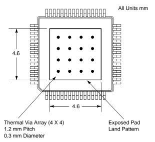
Figure 7. Recommended Thermal Land Pattern
