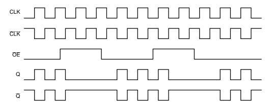
Figure 4. Output Enable (OE) Timing Diagram
