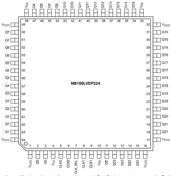
All  $V_{CC}$ ,  $V_{CCO}$ , and  $V_{EE}$  pins must be externally connected to appropriate Power Supply to guarantee proper operation. The thermally conductive exposed pad on package bottom (see package case drawing) must be attached to a heat–sinking conduit, capable of transferring 1.2 Watts. This exposed pad is electrically connected to  $V_{EE}$  internally.
