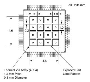
Figure 8. Recommended Solder Mask Openings
