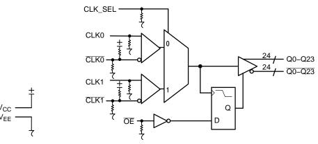
Figure 2. Logic Diagram
