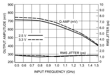
Figure 3. Output Amplitude (V<sub>OPP</sub>) versus Input Frequency and Random Clock Jitter (t<sub>JITTER</sub>)
