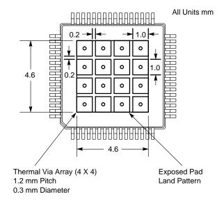
Figure 9. Recommended Solder Mask Openings
