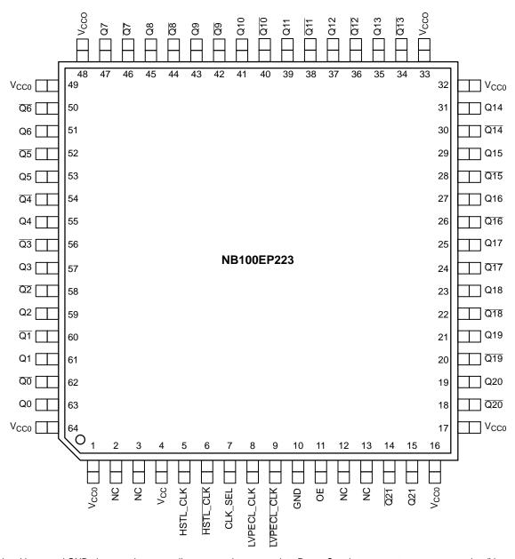
All  $V_{CC}$ ,  $V_{CCO}$ , and GND pins must be externally connected to appropriate Power Supply to guarantee proper operation ( $V_{CC} \neq V_{CCO}$ ). The thermally conductive exposed pad on package bottom (see package case drawing) is electrically connected to GND internally.
