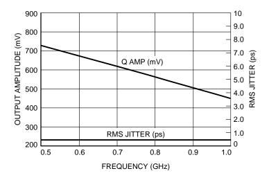
Figure 3. Output Frequency (F<sub>OUT</sub>) versus Output Voltage (V<sub>OPP</sub>) and Random Clock Jitter (t<sub>JITTER</sub>)
