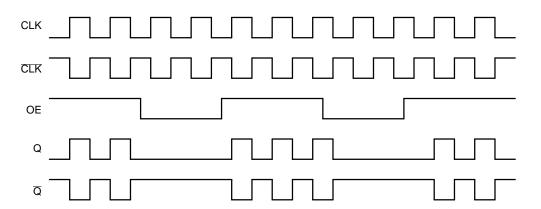
Figure 7. Output Enable (OE) Timing Diagram
