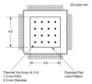
Figure 8. Recommended Thermal Land Pattern
