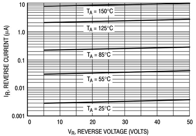
**Figure 3. Leakage Current**
