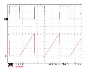
Figure 22. CT Voltage at Full Load Condition
