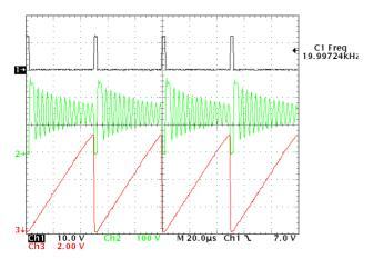
Figure 24. CT and Drain at Light Load
