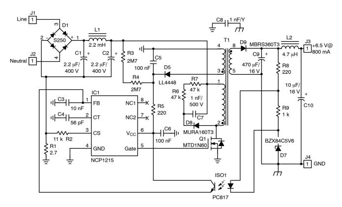
Figure 21. Adaptor Application Schematic
