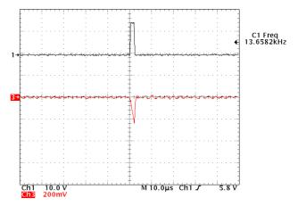
Figure 26. CS Pin at Light Load Condition
