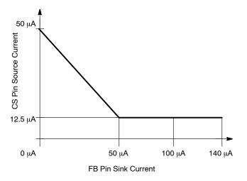
Figure 16. Current Sense Regulation Characteristic
