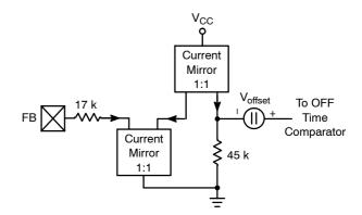
Figure 13. Feedback Loop - OFF Time Control
