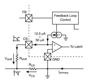
Figure 19. Primary Current Sensing
