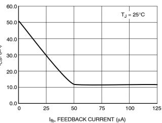
Figure 12. Current Sense Source Current vs. Feedback Current
