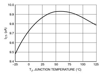
Figure 9. CT pin Source Current vs. Junction Temperature
