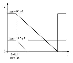
Figure 20. CS Pin Voltage
