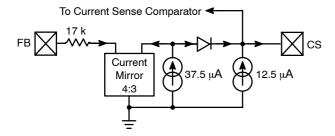
Figure 15. Feedback Loop - Current Sense Control
