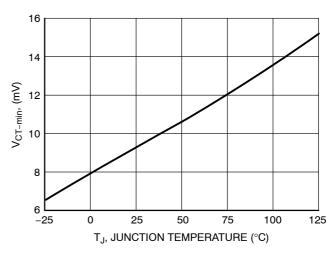
Figure 10. CT pin Threshold vs. Junction Temperature
