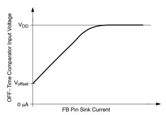
Figure 14. FB Loop Transfer Characteristic
