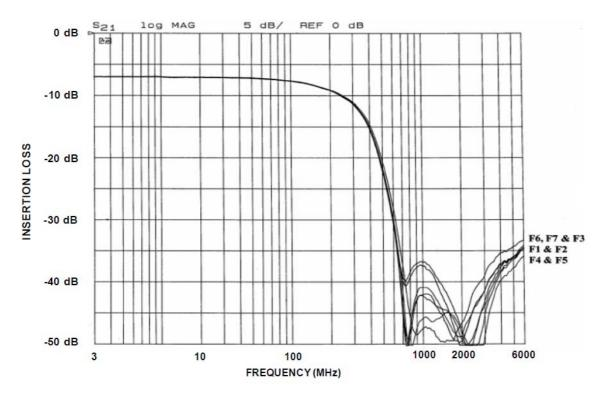
Figure 1. Typical Insertion Loss (Bias = 0 V,  $T_A$  = 25°C, 50  $\Omega$  Environment)
