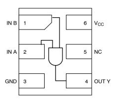
Figure 1. Pinout (Top View)
