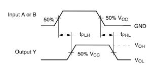
Figure 3. Switching Waveforms
