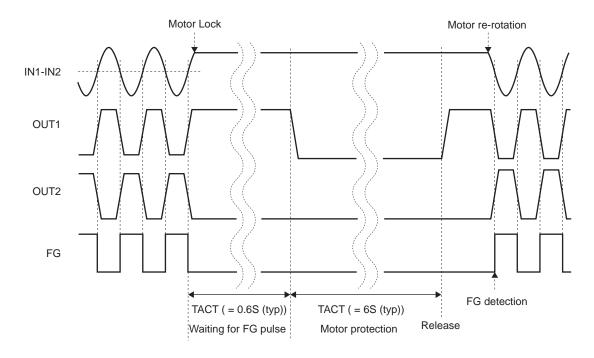
\* When motor protection is activated, both OUT1 and OUT2 output low level.
