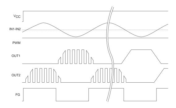
When the power supply is turned on, the standby release (quick start), and the lock protection is released, the start amends operation is done.
