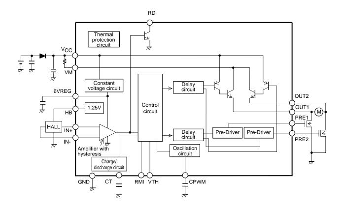
Sample Application Circuit 2 <no minimum speed setting, thermistor input>
