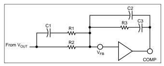
Figure 11: Two pole-two zero compensation network.
