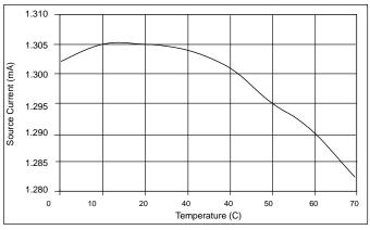
Figure 35: Error Amplifier Source Current vs Temperature.
