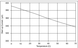
Figure 48: Start-up Current vs Temperature.
