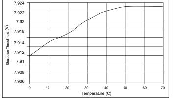
Figure 49:  $V_{\rm IN}$  Shutdown Threshold vs Temperature.
