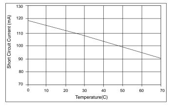
Figure 23:  $V_{\text{REF}}$  Short Circuit Current vs Temperature.
