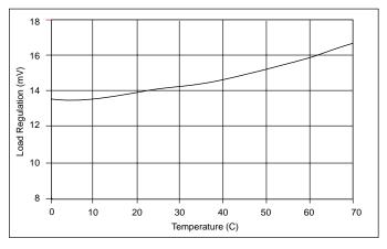
Figure 20: Load Regulation vs Temperature 1mA to 10mA.
