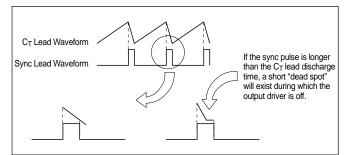
Figure 2a: Sync pulse duration vs. C<sub>T</sub> lead discharge time.
