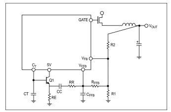
Figure 4: Artificial ramp components CC, C<sub>FFB</sub>, RR and R<sub>FFB</sub> must be provided for each channel if duty cycle for that channel exceeds 50%. Q1 and RE are common to both channels. DC voltage is shown supplied to  $V_{FFB}$  through the  $V_{FB}$  resistor divider.
