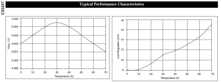
Figure 19: V<sub>REF</sub> vs Temperature, 1mA Load.
