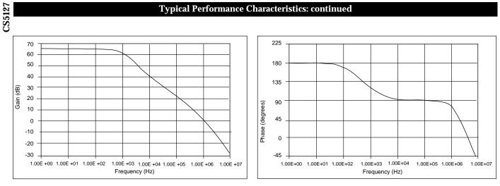
Figure 31: Error Amplifier Gain vs Frequency.
