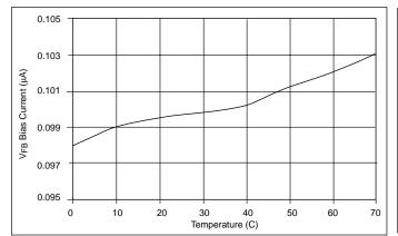
Figure 33:  $V_{FB}$  Bias Current vs Temperature.
