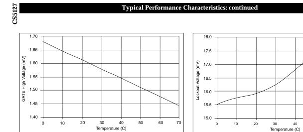
Figure 43: GATE High Voltage (100mA) vs Temperature.
