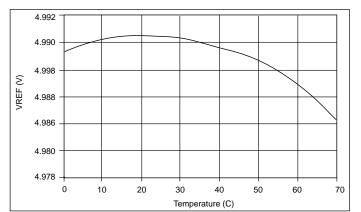
Figure 21:  $V_{REF}$  vs Temperature, 10mA Load.
