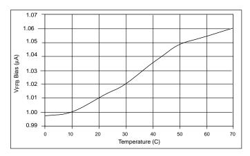
Figure 39: V<sub>FFB</sub> Bias Current vs Temperature.
