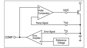
Figure 1: V<sup>2<sup>TM</sup></sup> control diagram.
