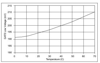
Figure 42: GATE Low Voltage (100mA) vs Temperature.
