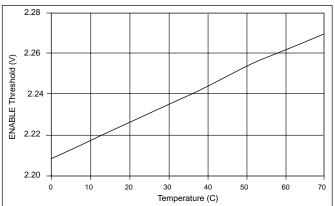
Figure 40: ENABLE Threshold vs Temperature.
