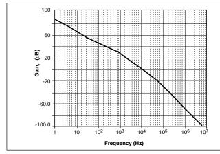
Figure 9: Bode plot of gain response for compensated voltage mode system.
