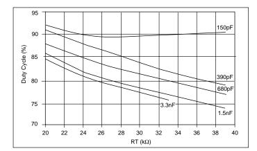
Figure 27: Oscillator Duty Cycle vs  $C_T$ ,  $R_T$  ( $V_{IN}$  = 12V, T = 25C).
