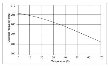
Figure 26: Oscillator Frequency vs Temperature. C<sub>T</sub> = 330pF, R<sub>T</sub> =27k
