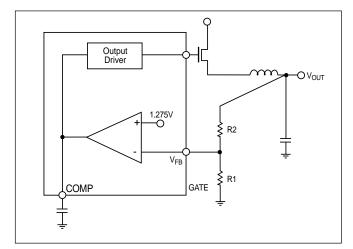
Figure 3: Feedback resistor divider.
