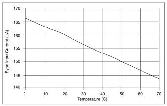
Figure 29: SYNC Input Current vs Temperature (V<sub>SYNC</sub> = 2.4V).
