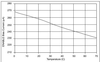
Figure 41: ENABLE Bias Current vs Temperature.
