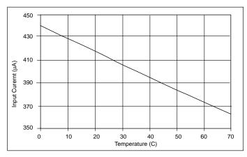
Figure 32: SYNC Input Current vs Temperature (V<sub>SYNC</sub> = 5V).
