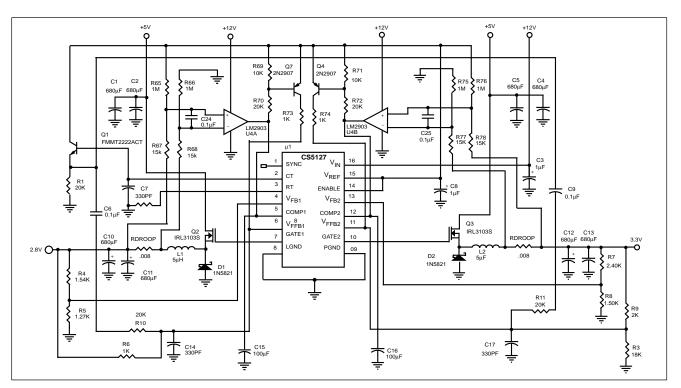
Figure 17: 200kHz, V<sup>2TM</sup>, 5V/12V input, 2.8V@ 7A and 3.3V @ 7A outputs with current limit.
