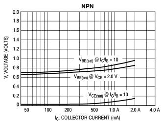
Figure 3. MPS650, MPS651 On Voltages
