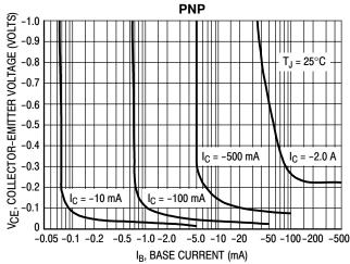
Figure 6. MPS750, MPS751 Collector Saturation Region
