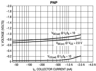
Figure 4. MPS750, MPS751 On Voltages
