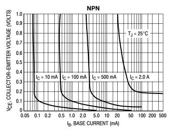
Figure 5. MPS650, MPS651 Collector Saturation Region
