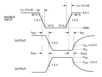
Figure 6. Enable/Disable Delays
