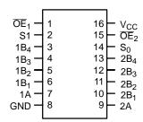
Figure 1. 16-Lead Pinout
