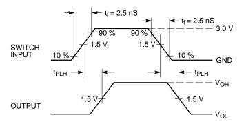
Figure 5. Propagation Delays
