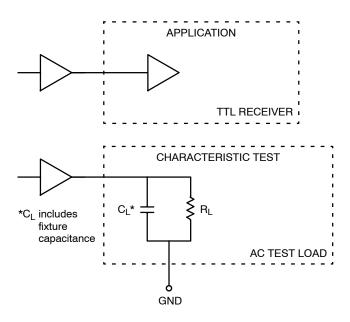
Figure 1. TTL Output Loading Used for Device Evaluation
