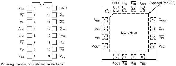
For PLCC pin assignment, see the Pin Conversion Tables.
