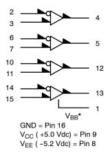
$^*V_{BB}$  to be used to supply bias to the MC10H125 only and bypassed (when used) with 0.01  $\mu F$  to 0.1  $\mu F$  capacitor to ground (0 V).  $V_{BB}$  can source < 1.0 mA.
