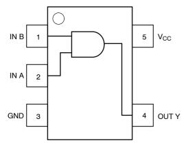
Figure 1. Pinout (Top View)
