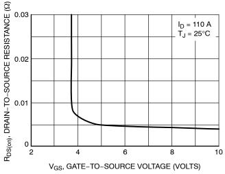
Figure 3. On–Resistance versus Gate–to–Source Voltage
