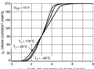
V<sub>GS</sub>, GATE-TO-SOURCE VOLTAGE (VOLTS) Figure 2. Transfer Characteristics
