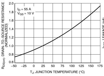
Figure 5. On–Resistance Variation with Temperature
