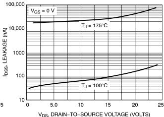
Figure 6. Drain-to-Source Leakage Current versus Voltage
