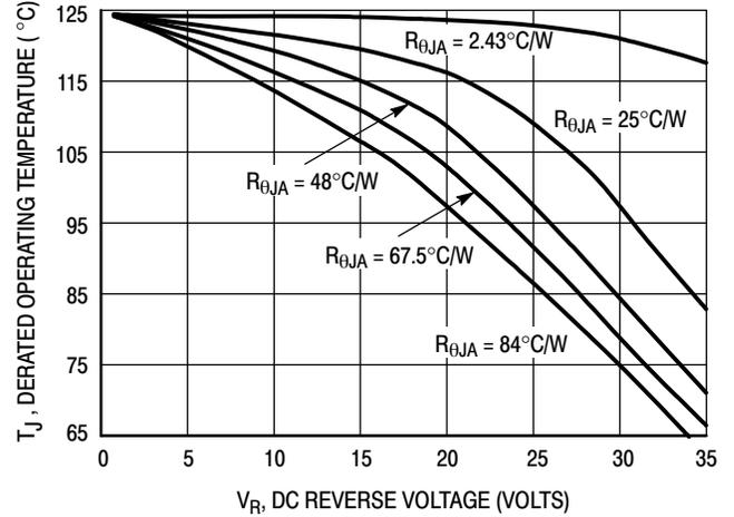
Figure 8. Typical Operating Temperature Derating Per Leg \*
