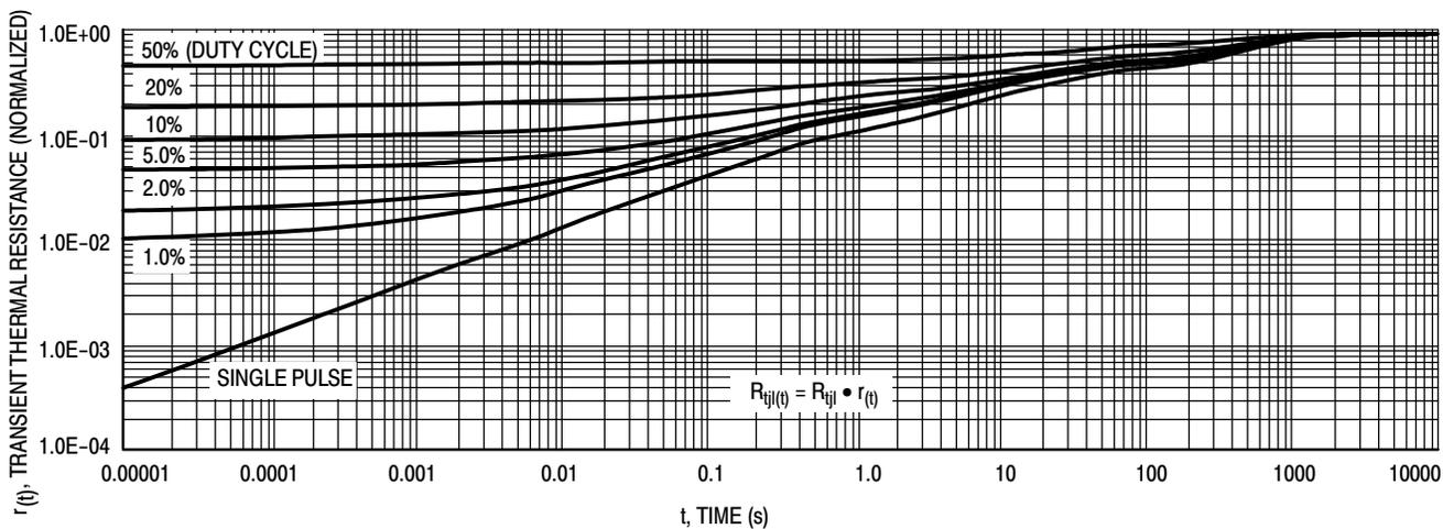
Figure 10. Thermal Response Junction to Ambient (Per Leg)
