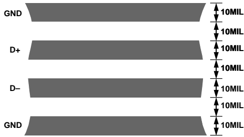
Figure 19. Arrangement of Signal Tracks
