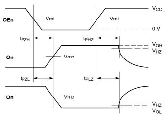
WAVEFORM 1 – PROPAGATION DELAYS, SETUP AND HOLD TIMES  $t_B = t_F = 2.5$  ns, 10% to 90%; f = 1 MHz;  $t_W = 500$  ns
