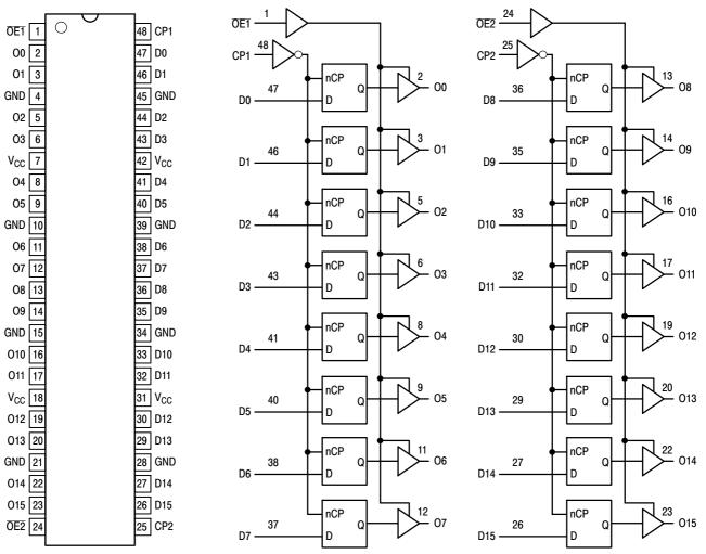
Figure 1. Pinout: 48-Lead (Top View)
