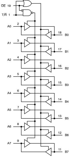
Figure 2. Logic Diagram
