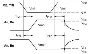
**WAVEFORM 1 – PROPAGATION DELAYS**  $t_{B} = t_{F} = 2.5 \text{ ns}, 10\% \text{ to } 90\%; f = 1 \text{ MHz}; t_{W} = 500 \text{ ns}$
