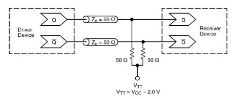
Figure 17. Typical Termination for Output Driver and Device Evaluation (See Application Note AND8020/D – Termination of ECL Logic Devices.)
