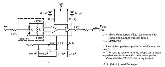
Tank Circuit Option #1, Varactor Diode
