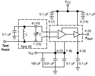
L = Micro Metal torroid #T20-22, 8 turns #30 Enameled Copper wire (@ 40 nH)
