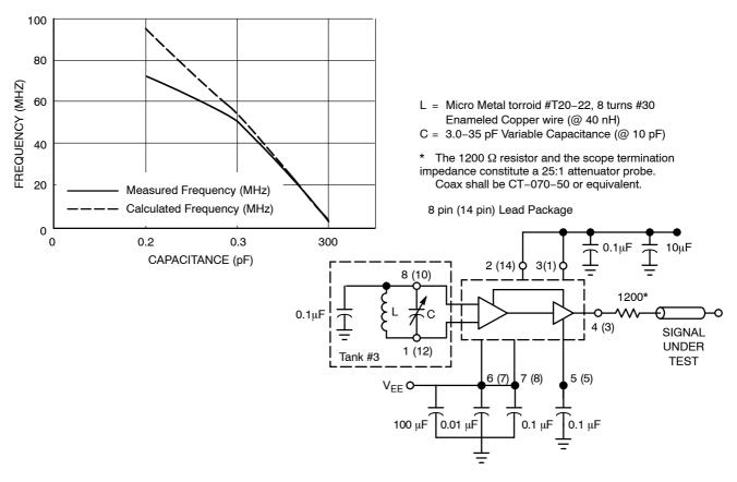
Figure 7. High Frequency Plot
