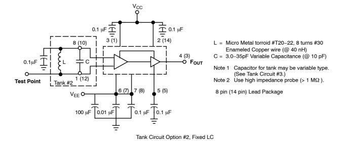
Figure 3. Typical Test Circuit with Alternate Tank Circuits
