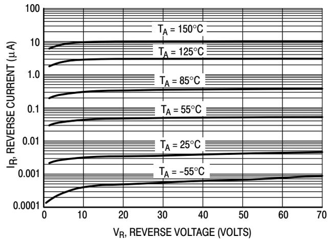
Figure 2. Leakage Current
