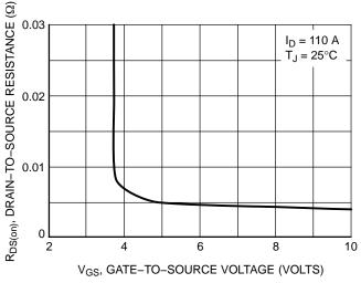
Figure 3. On–Resistance versus Gate–to–Source Voltage
