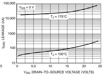
Figure 6. Drain-to-Source Leakage Current versus Voltage
