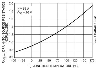
Figure 5. On–Resistance Variation with Temperature
