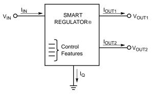
Figure 24. Dual Output Regulator With Key Performance Parameters Labeled.
