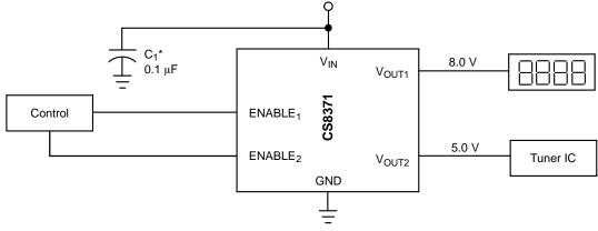
\* C1 is required if the regulator is far from the power source filter.
