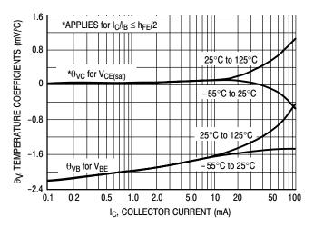
Figure 12. Temperature Coefficients
