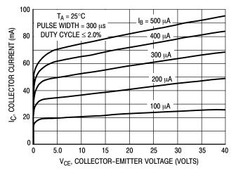
Figure 10. Collector Characteristics
