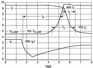
Figure 18. Dynamic Saturation Voltage Measurements
