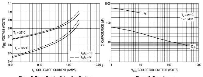
Figure 5. Base–Emitter Saturation Region
