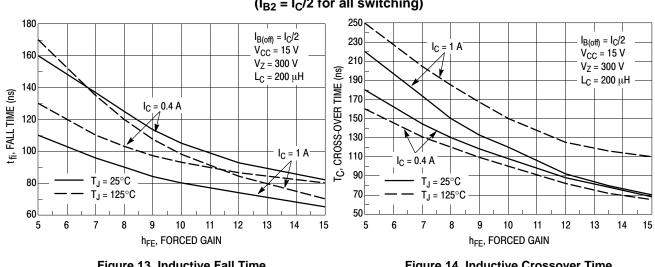
**TYPICAL SWITCHING CHARACTERISTICS**  $(I_{B2} = I_C/2 \text{ for all switching})$
