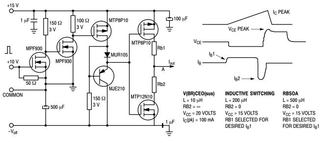
Table 1. Inductive Load Switching Drive Circuit
