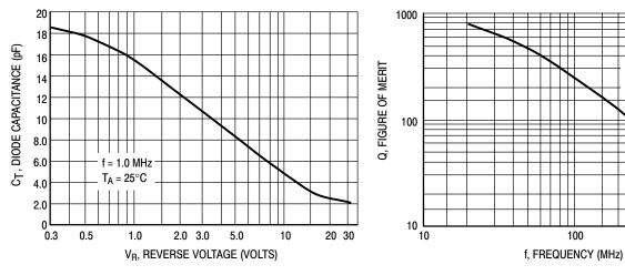
Figure 1. Diode Capacitance
