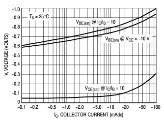
Figure 2. "Saturation" and "On" Voltages
