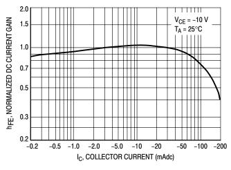
Figure 1. Normalized DC Current Gain
