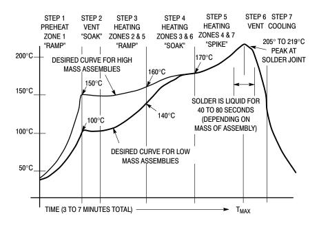
Figure 12. Typical Solder Heating Profile
