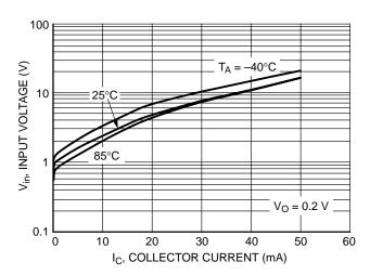
Figure 11. Input Voltage versus Output Current
