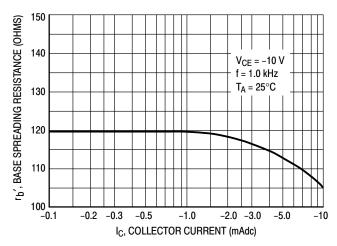
Figure 6. Base Spreading Resistance
