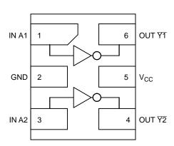
Figure 1. Pinout (Top View)
