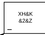
Pin#1 Identifier UQFN16 (MicroMLP) (Top View)
