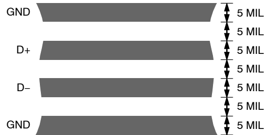
Figure 34. Typical Arrangement of Signal Tracks
