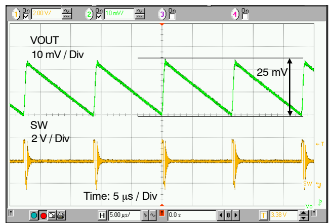
Figure 14. Output Ripple Voltage in PFM Mode ( V_{IN} = 3.6\text{ V} , V_{OUT} = 1.8\text{ V} , I_{OUT} = 10\text{ mA} , L = 1\text{ }\mu\text{H} , C_{OUT} = 10\text{ }\mu\text{F} )
