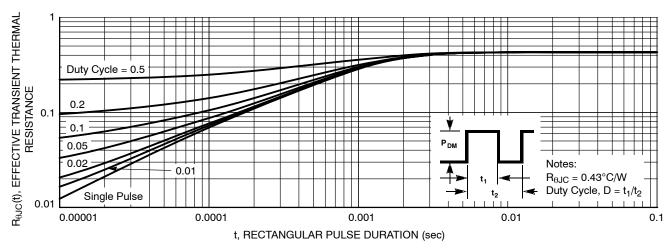
Figure 13. Transient Thermal Impedance
