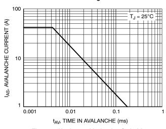
Figure 9. Unclamped Inductive Switching Capability
