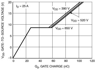
Figure 7. Gate-to-Source Voltage vs. Total Charge
