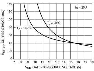
Figure 4. On-Resistance vs. Gate-to-Source Voltage
