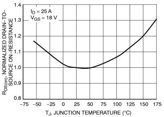
Figure 3. On–Resistance Variation with Temperature
