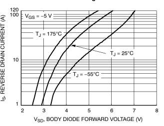
Figure 6. Diode Forward Voltage vs. Current
