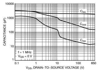
Figure 8. Capacitance vs. Drain-to-Source Voltage
