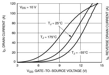
Figure 5. Transfer Characteristics
