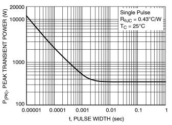
Figure 12. Single Pulse Maximum Power Dissipation
