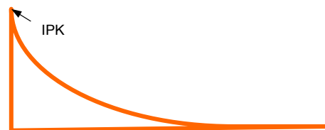
Figure 26. Input Charge Inrush Current
