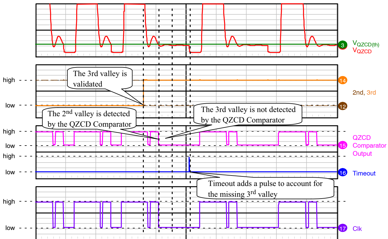
Figure 22. Timeout Operation with a Missing 3 rd Valley
