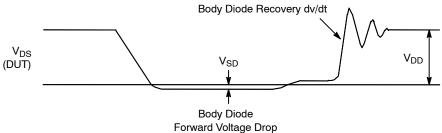
Figure 20. Peak Diode Recovery dv/dt Test Circuit & Waveforms
