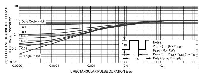
Figure 16. Transient Thermal Response
