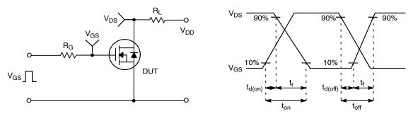
Figure 18. Resistive Switching Test Circuit & Waveforms
