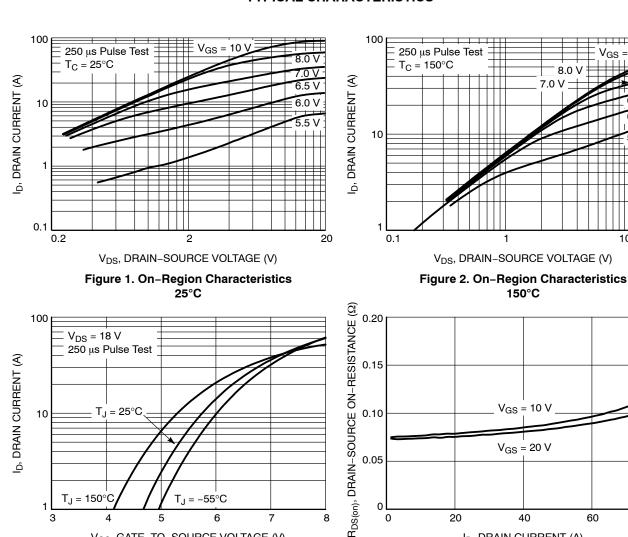
V<sub>GS</sub>, GATE-TO-SOURCE VOLTAGE (V) Figure 3. Transfer Characteristics
