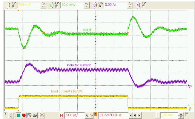
Figure 28. Load Transient, 3.6 V_{IN} , 1.2 V_{OUT} , 1.5–6 A, 100 ns Edge, C_{OUT} = 4 \times 22\ \mu\text{F}
