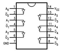
Figure 1. Connection Diagram
