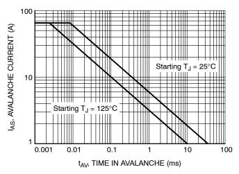
Figure 15. Unclamped Inductive Switching Capability
