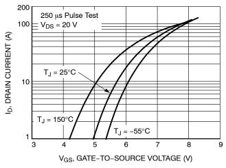
Figure 3. Transfer Characteristics
