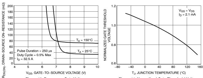
Figure 13. R<sub>DS(ON)</sub> vs. Gate Voltage
