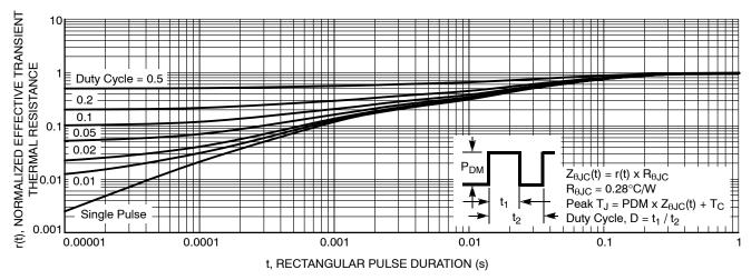
Figure 16. Transient Thermal Response Curve
