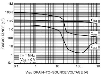
Figure 6. Capacitance Characteristics
