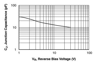
Figure 2. Typical Junction Capacitance
