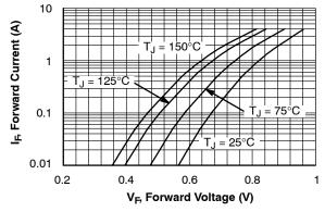
Figure 4. Typical Forward Characteristics
