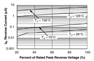
Figure 3. Typical Reverse Characteristics
