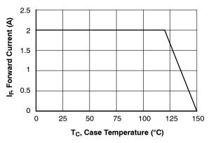
Figure 1. Forward Current Derating Curve
