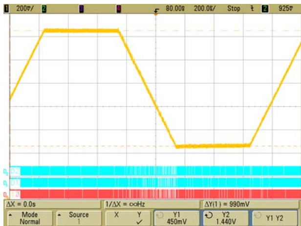
Figure 8. DVID Waveform (by VTT, 0.5 V-1.5V) 1-Vo D0~D2-PWM1~3
