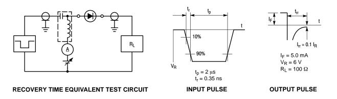
Figure 5. Reverse Recovery Time Test Circuit for the DAP202U
