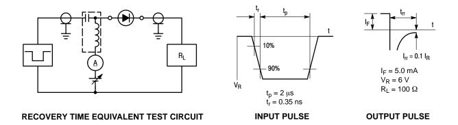
Figure 4. Reverse Recovery Time Test Circuit for the DAP222
