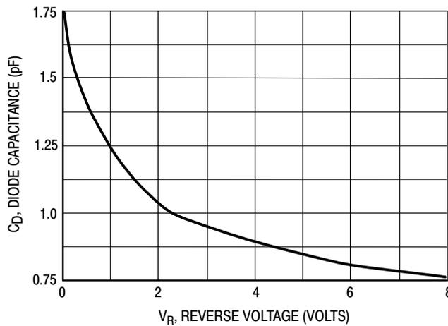
Figure 3. Diode Capacitance
