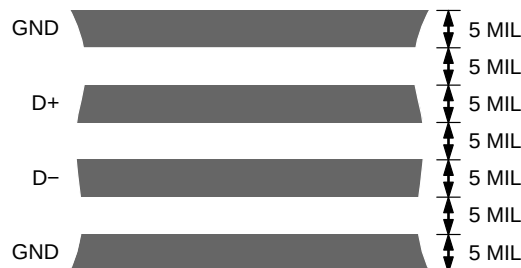
Figure 34. Typical Arrangement of Signal Tracks
