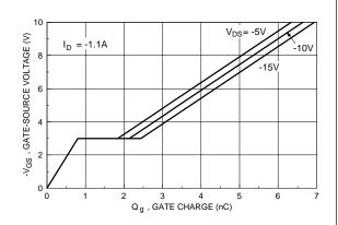
Figure 10. Gate Charge Characteristics.
