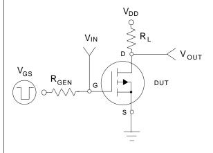
Figure 11. Switching Test Circuit.
