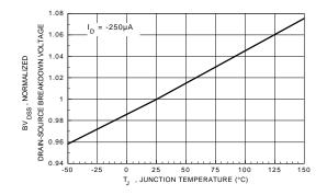
Figure 7. Breakdown Voltage Variation with Temperature.
