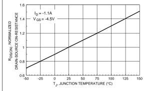
Figure 3. On-Resistance Variation with Temperature.
