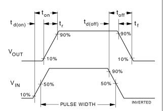
Figure 12. Switching Waveforms.
