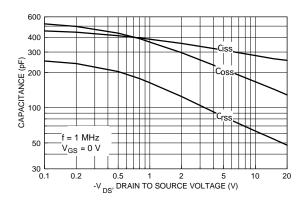
Figure 9. Capacitance Characteristics.
