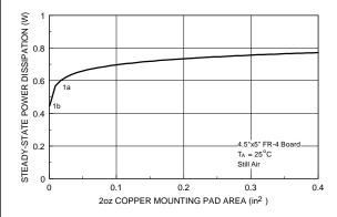
Figue 15. SuperSOT™-3 Maximum Steady-State Power Dissipation versus Copper Mounting Pad Area.
