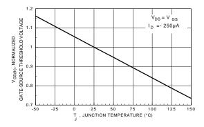
Figure 6. Gate Threshold Variation with Temperature.
