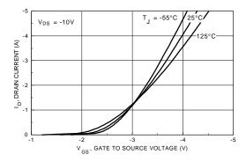
Figure 5. Transfer Characteristics.
